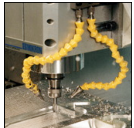
Cavity milling with HSC-technology, 2-nozzles Unilube MicroLubricationSystem
