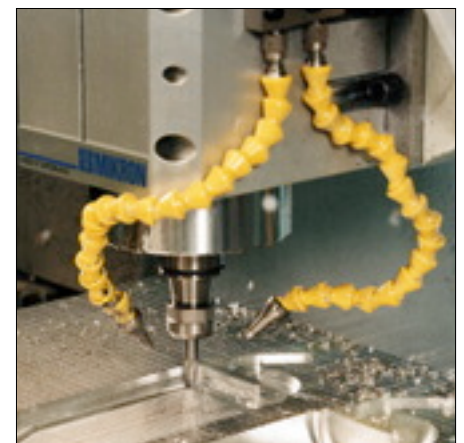
Cavity milling with HSC-technology, 2-nozzles Unilube MicroLubricationSystem
