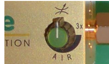
Fig. 16: Air regulation – factory setting open by 1 turn
