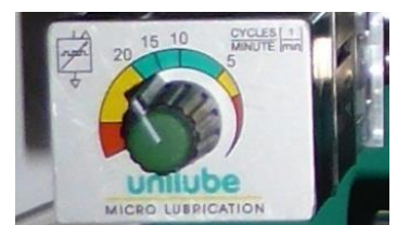
Fig. 14: Pneumatic Pulse Generator – factory setting 20 cycles / min
