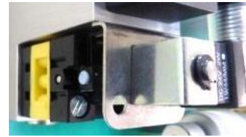
Fig. 15: Electric Pump Control Valve – cycles from control system
