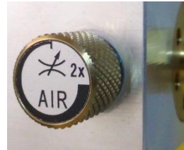
Fig. 17: Air regulation – factory setting open by 1 turn
