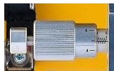
Fig. 14: Micrometer screw – factory setting 0.5 turns
